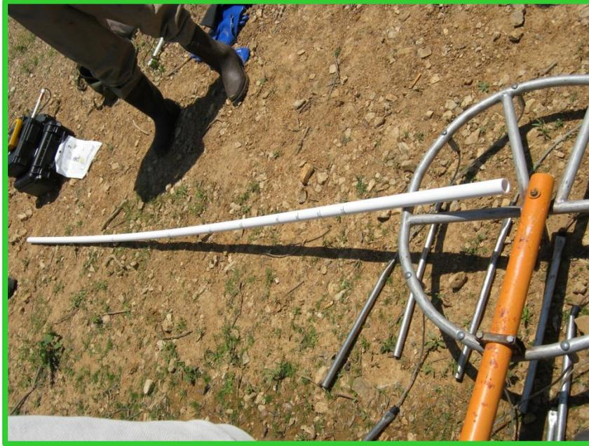
At pre-determined distances and/or at voltage gradients of interest, record voltage gradient at distance and direction from an electrode. Direction can be straight-ahead, directly lateral, aft, or some oblique angle.
