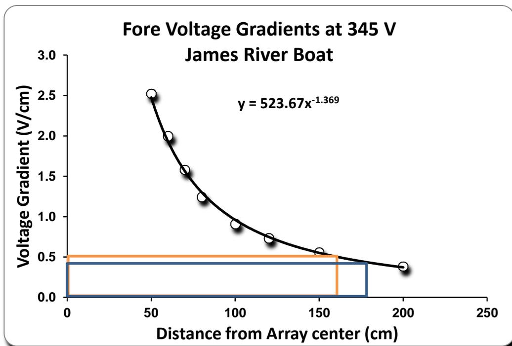
$$\text{Distance from anode center to 0.4 V/cm point} = \left(\frac{0.4}{523.67}\right)^{\frac{1}{-1.369}} = 189 \text{ cm}$$
