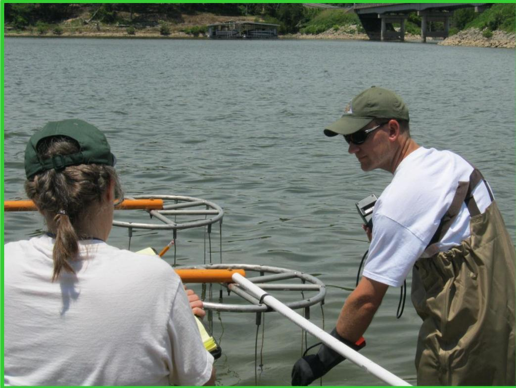
*Taking a measurement:* place the bottom of the probe in the water to a consistent depth (e.g., 50% of submergence distance of droppers). If using DC or PDC, orient the anodic (red) end of the probe toward the anode or the cathodic probe end toward the cathode. Rotate the probe slowly until a maximum reading is obtained. If using a 1 cm probe electrode separation distance, then directly read V/cm from the multimeter display.
