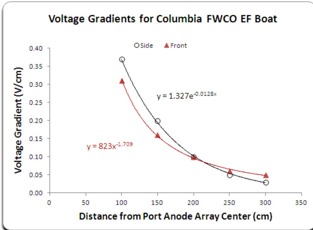
In the above graph example of a boat boom dropper array electric field, a forward (Front) and lateral (Side) pattern is plotted and fit with exponential prediction equations. Prediction equations allow estimation of distance from electrode center or surface for voltage gradients of interest (as immobilization threshold values). For example, the following graph and re-arranged equations indicate the distance from anode center that the 0.4 and 0.5 V/cm gradients occur.
