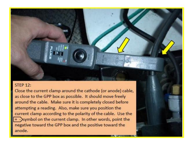
Record the measurement in millivolts. Then take that value and divide by the current clamp scale (usually 10 mV/amp or 100 mV/amp; in this case, 10 mV/amp) to get the amperage. For example, a reading of 342 mV peak would translate to 342/10 = 34.2 peak amps.
