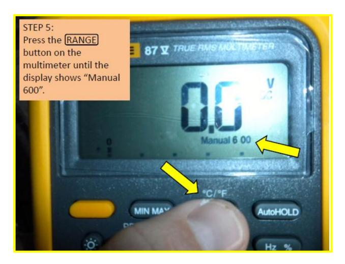
This model has an auto-range voltage scaling capability; however, it is better to set the meter in manual mode to the 600 V range since higher voltages are used. Another safety note is that the "do not exceed" rating (CAT II or CAT III) of this particular meter is 600 Vrms.
