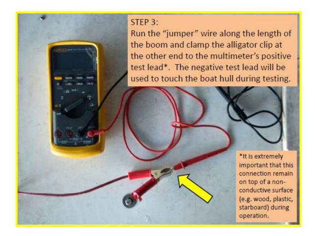
As noted, this connection constitutes a potential hazard. The safest and recommended approach is to have an unbroken test lead long enough to reach from the multimeter to the boom.
