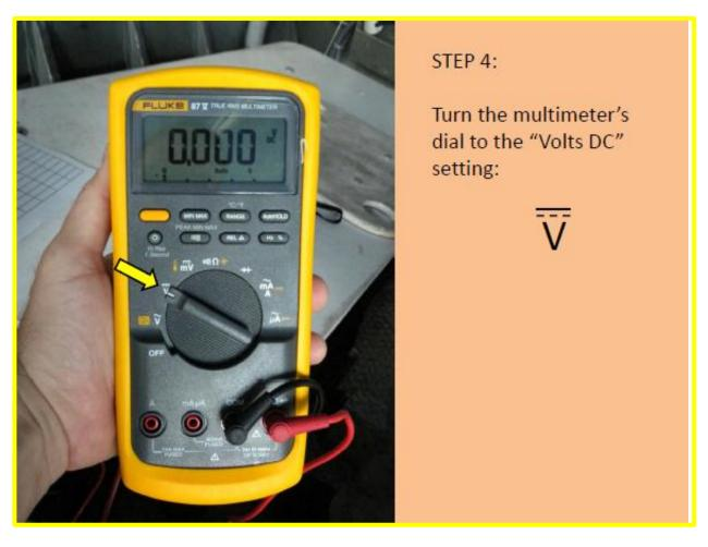
This setting is for measuring DC or PDC. For measuring AC, the dial would need to be set to  $V^{\sim}$ .
