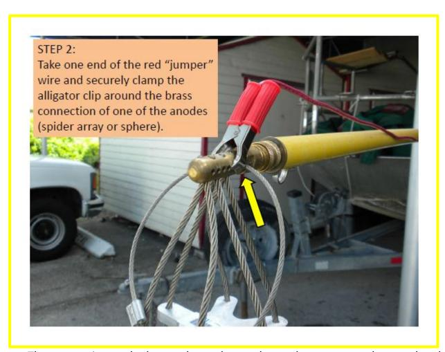
The connection to the boom electrodes can be made anyway on the metal end, as on one dropper. The important thing is to make a good, secure electrical connection.
